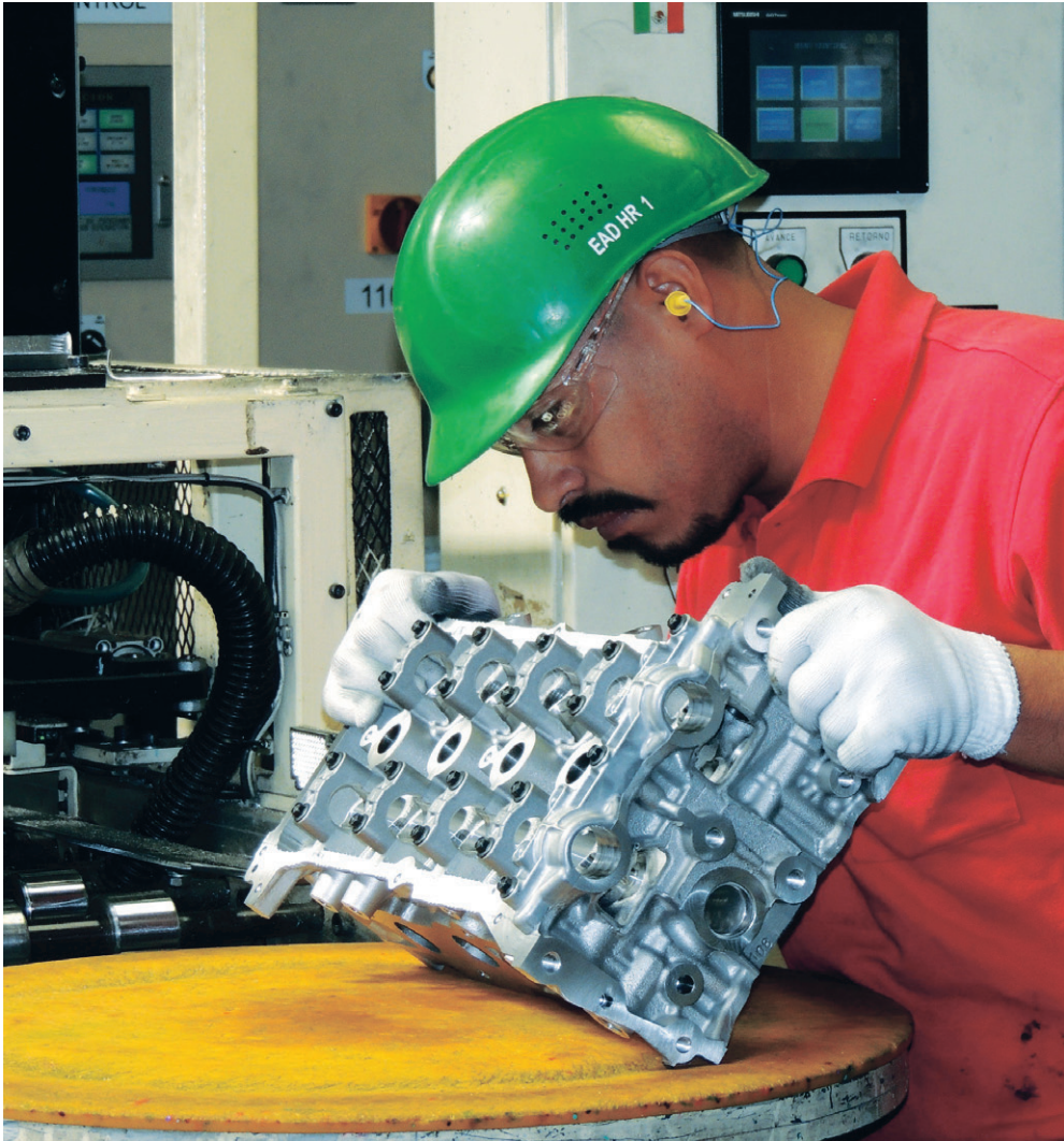
NMEX checkman is performing the final inspection of the cylinder head for a Micra engine. He is on the lookout for burrs and casting concerns.
