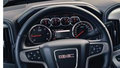
The 2014 Sierra's new gauge cluster with six gauges and a 4.2-inch color Driver Information Center showing vehicle status information, a trip computer and other information, such as radio and navigation.
