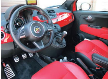
The bright and cheery interior of the Abarth also contains a number of features not found on other 500 models like high back bucket seats, three-spoke leather wrapped steering wheel, analog turbo-boost gauge and aluminum pedal pads and door sill plates.
