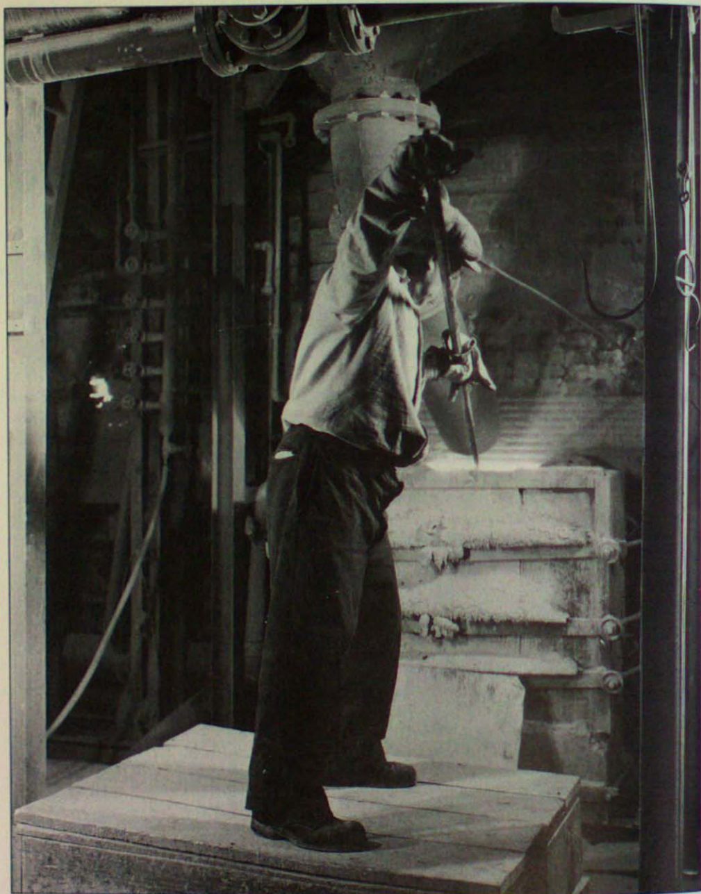
STIRRING A BATCH. Production at Wallaceburg's glass factory began in 1894. Over the years, every conceivable type of container or ware has been produced at the hands of local glass staff. A worker close to the heat, stirs up another molten glass concoction. (Wallaceburg Museum Collection.)
